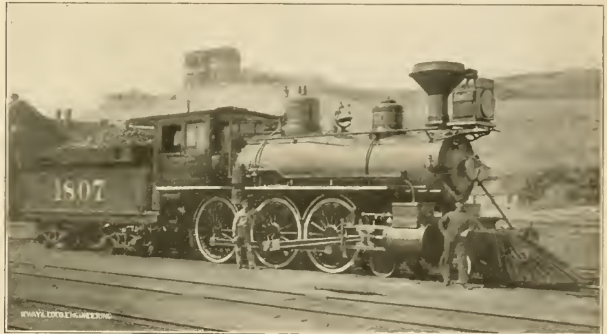
A "WESTERN," BUILT AT THE UNION PACIFIC SHOPS, OMAHA—THE MODERN POWER FOR MOVING FREIGHT ON THE PRAIRIE.
